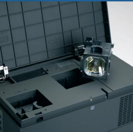
▲ The LX900 new dual lamp design provides high brightness and increased uniformity even in a single lamp mode.
