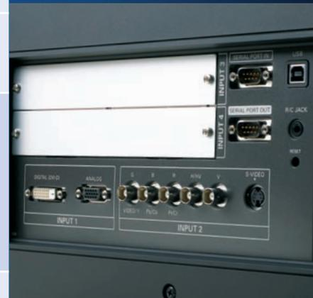
▲ The LX900 offers input flexibility by providing two option board slots to allow for additional signal connectivity from a variety of option cards.
